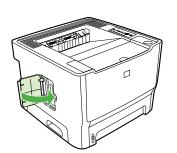
Close the DIMM access door, reconnect all cables and cords, then turn the power switch on.
